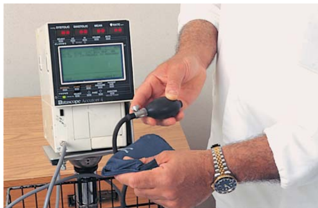
Figure 24-5. The automatic blood-pressure monitor reports systolic, diastolic, and mean blood pressure. (Photo © B. Proud.)
